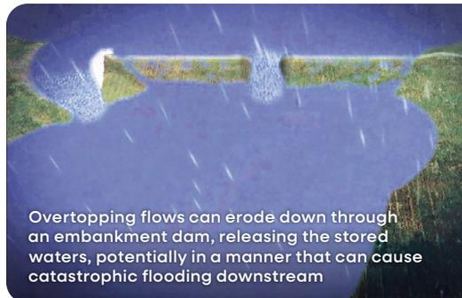
Overtopping flows can erode down through an embankment dam, releasing the stored waters, potentially in a manner that can cause catastrophic flooding downstream
