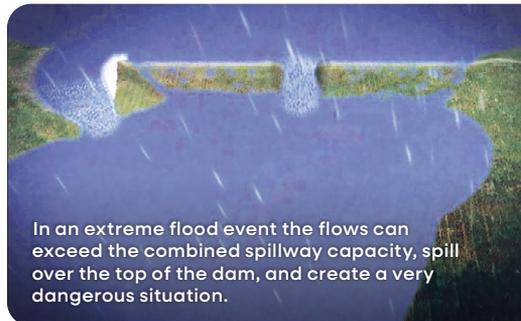
In an extreme flood event the flows can exceed the combined spillway capacity, spill over the top of the dam, and create a very dangerous situation.
